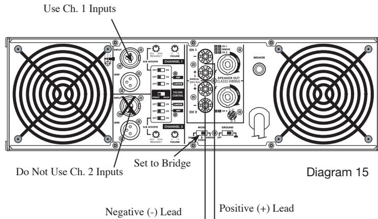
Use the two red terminal from the banana jacks to power a subwoofer speaker in mono-bridge mode.
