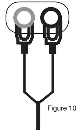
**SPEAKON ASSEMBLY:** You will need a pair of Neutrik Speakon® NL4FC connectors. You will also need high-quality two or four conductor speaker cable, a pair of needle-nosed pliers and a 1.5-mm Allen key to assemble the Speakon connectors to your speaker wire. To assemble the Neutrik Speakon NL4FC connector, complete the following steps:
